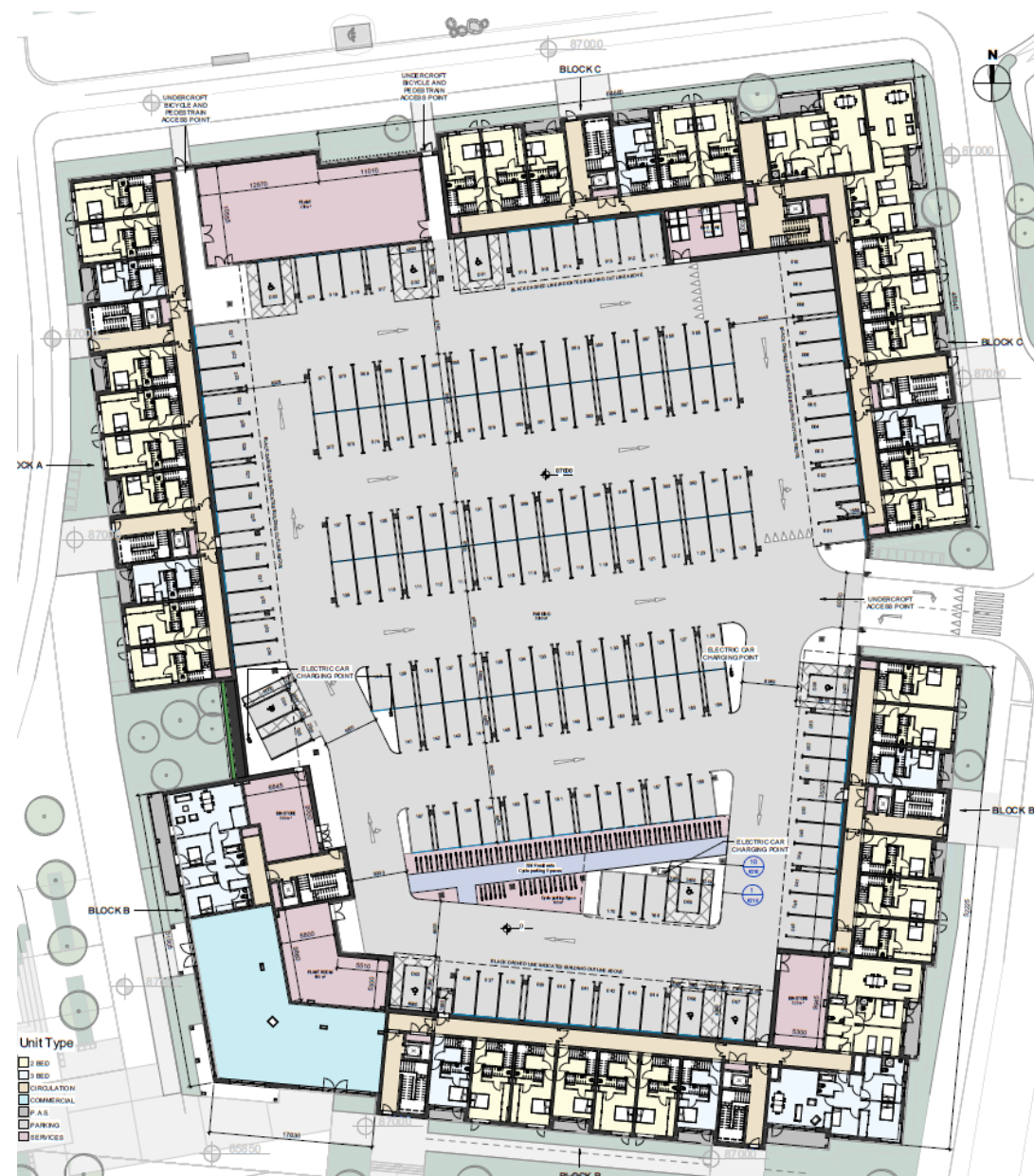
Figure 6.9: Undercroft car parking at ground floor level
