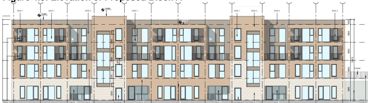
Figure 4.3: Elevation of Proposed Block A
