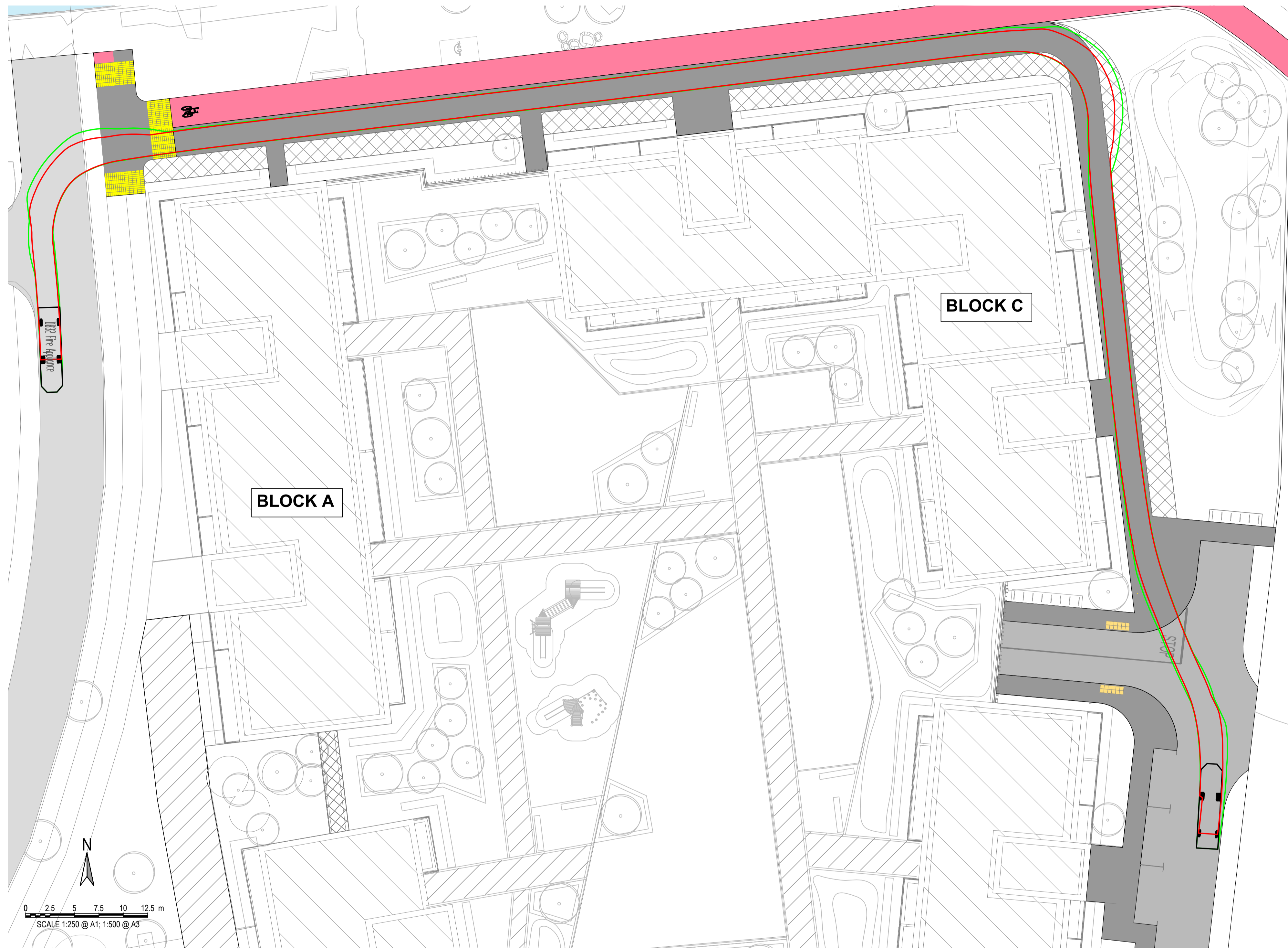
AUTOTRACK LAYOUT FOR FIRE APPLIANCE
